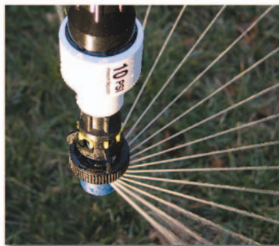
The Part-Circle LDN distributes water away from wheel tracks. (For use on rigid drops.)
